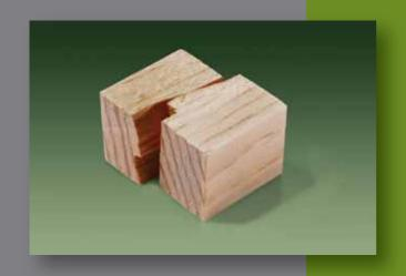
The laminated bonds are cut into block shear specimens 2" width and 1 34" in length. Laminated bonds are tested in shear by compression loading. The strength required to break the block as well as the percentage of wood failure is recorded.
