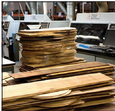
Woodsets await cutting and assembly. Mahogany is the preferred species for necks and pegheads.
